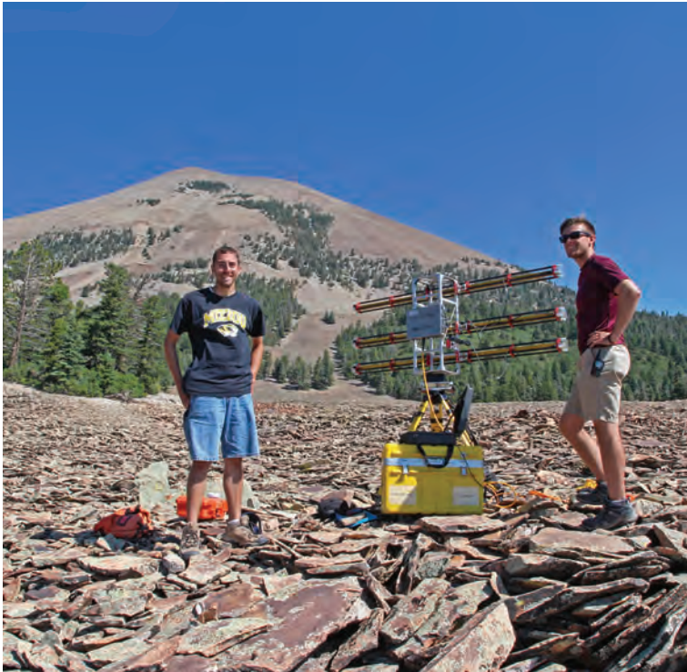
Dan Clapp and David Nymberg operating the ground-based radar interferometer to measure movement of a rock glacier on Mt. Mestas (Colorado) as part of Dan's undergraduate research, August 2017.
