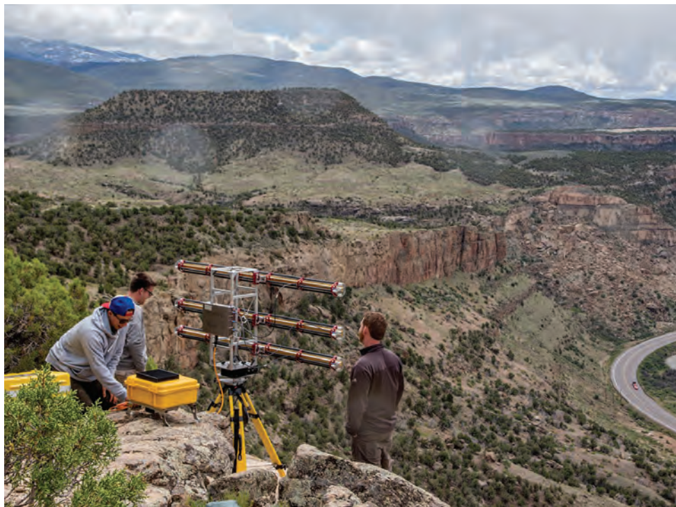
From left: Charlie Miles, Dan Clapp and Kelly Hickcox surveying the Debeque Canyon (Colorado) landslide (background) with the ground-based radar as part of Kelly's thesis research, May 2017.
