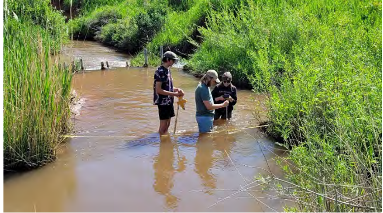
Matthew Mollica (UT - Chattanooga), Sam Pritchett (MU) and Teaching Assistant Emily Edwards collecting flow velocity measurements for streamgaging Red Canyon Creek.
